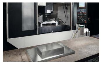
In its own milling shop, ACL produces all-aluminium housings, which have an excellent thermal conductivity and thus, as passively cooled housings, enable a long life of the electronic components.
