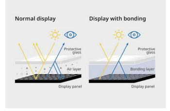
Optical bonding minimises distorted light refractions, prevents soiling and minimises the risk of falling splinters falling in the event of damage.
