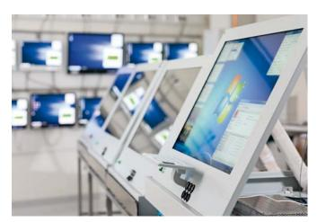
The OR-CONSOLE® - like all ACL devices - undergoes a comprehensive quality check before delivery. In addition to a visual inspection and an intensive functional test, all integrated electronic components are subjected to a documented stress test to guarantee the durability of the device.
