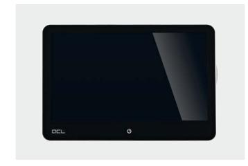
With a total weight of only 2.4 kg, the Bedside Terminal can be flexibly installed directly at the patient's bed and connected to the modern media world. Each patient can therefore decide individually at any time what he or she wants to hear, see or read. The terminal offers an integrated loudspeaker, a headphone connection, USB port and smart card reader.
